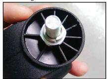
Place a spring washer over the screw bolt on the wheel.
