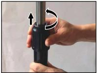
4. Rotate the grip counter clockwise to loosen completely and remove from top of pole.
