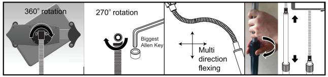
Use the biggest Allen key to tighten and loosen the gooseneck connection screw, adjusting ease of rotation in the tablet holder.
