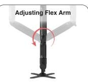
Twist the screw knob of the arms counter-clockwise to release the connection. Adjust the arms to your favorite position and then tighten the screw knob clockwise.
