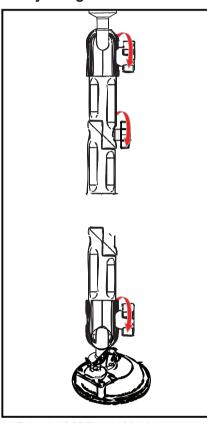
1. Twist the SCREW KNOB of the arms counter clockwise to release the connection
