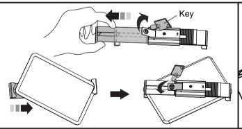
1. Insert key into lock at back of holder. Turn counterclockwise to unlock, then slide to open. Insert tablet against fixed end, then slide down to hold tight. Turn key clockwise to lock.
