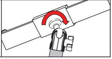
2. Loosen ball socket joint to rotate tablet to desired orientation, then tighten ball socket again.
