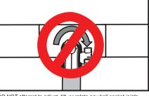
DO NOT attempt to adjust, tilt, or rotate any ball socket joints while it is fully tightened. Any such action will result in possible damage and loss of integrity of product functioning at full capacity. Manufacturer will not be responsible for any such actions by any person.
