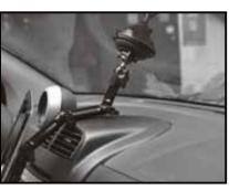
Keep the ARM closed to the central console will reduce the vibration
