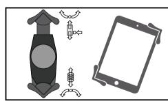
1. Press quick release button on side of tablet holder to release the adjustable end. Insert tablet corner against the spring arm, then push adjustable arm down against opposite corner. Be sure it is as snug
