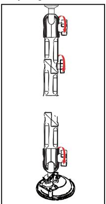
1. Twist the SCREW KNOB of the arms anticlockwise to release the connection.
