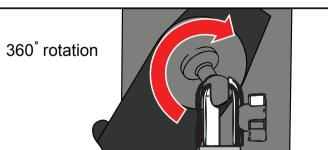
adjustable end. Insert tablet corner against the spring arm, then push custom viewing angles. adjustable arm down against opposite corner. Be sure it is as snug as possible.
