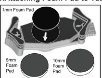
Select the appropriate foam pad according to the thickness of your tablet (or tablet in its case), then press adhesive side into center of the tablet holder
