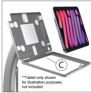
4B. Place your tablet device inside the tray (C). **Tablet only shown for illustration purposes, not included.
