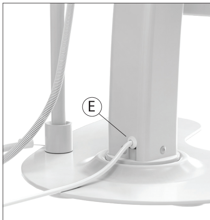
6B. Slide protectors over the cable, then fish the wire out the other end as shown.
