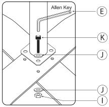
1A. Assemble all the different components illustrated to the left. Insert the screw bolt (K) through all of them in the corresponding order as shown. Using your hand to initially rotate in the screw while your other hand is holding the hex nut (I).
