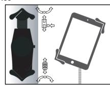
Press button on side of tablet holder to slide open. Insert your tablet against spring arm, then slide other end back down.
