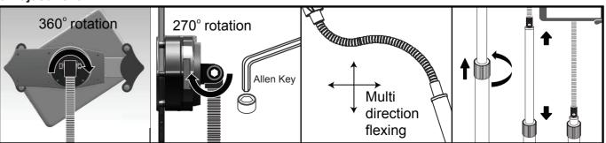
Use the Allen key to tighten and loosen the gooseneck connection screw, adjusting ease of rotation in the tablet holder.
