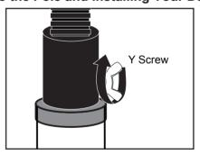
Turn the Y screw clockwise to tighten the connection.
