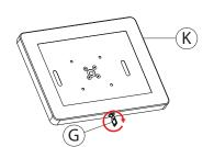
4A. Lock or unlock your tablet enclosure (K) with security key (G) as shown. Make sure to do a full 360 degree rotation before removing.
