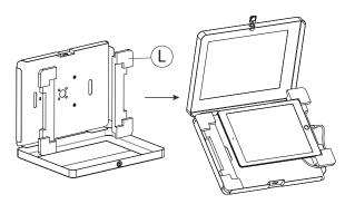
4B. Find the appropriate size foam padding / sheet (L) for the device you wish to use. Make sure the device is compatible for the enclosure before starting. Lay in device and connect any cables/cords as needed. There are sticker notes at the corners to identify which device is compatible
