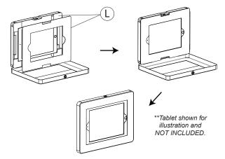
4C. If needed, lay-in correct included masking insert. The foam insert is to block and excess space and make a seamless fit for smaller tablets Close and lock enclosure afterwards and you're set.
