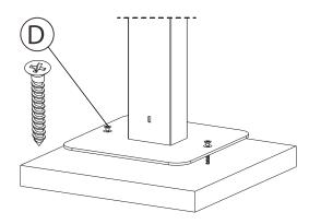
4A. Place the kiosk on top of desired surface, then rotate in screws (F) with a screwdriver tool (not included) until securely tightened.
