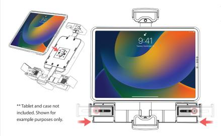
3D. Insert a tablet with compatible case attached. Make sure the two adapters are aligned. Once you insert the tablet with case, it will slide down to let you know it is in the right location. Then, retract the X-direction arms to find the right distance. Remove tablet and use screwdriver to tighten the desired position.
