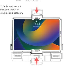
3E. Re-insert the tablet with compatible case. Using your arms, retract the holder in the Y-direction and Z direction until securely fitted.
