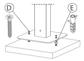
4B. Insert the anchors into the surface's pre-drilled holes then align kiosk base mounting holes to the pre-drill hole locations. Rotate in screws (F) from above with screwdriver tool (not included) until securely tightened.
