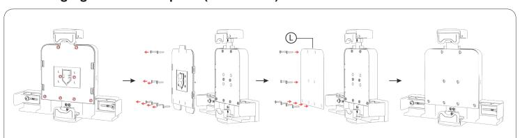
8A. Remove (8) front screws usign a screwdriver (not included) as shown above. Replace front place with component (L) and rotate in screw until securely tightened.
