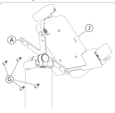
2A. Align VESA holes of Kiosk (A) to the VESA holes on the back of the holder (J). Using included tool (H), rotate in 4 screws (G) until securely fastened.
