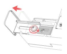
3B. Locate the X-direction holder arms. Using a screw driver (not included), rotate until loosened, then extend arms outwards.
