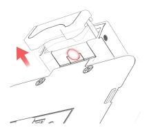
3C. Locate the Z-direction grip arms. On the inside for both the top and bottom, there is a circular button. Press down to loosen the grip arms and extend outwards.
