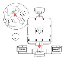
3A. First, make sure the holder is in unlocked position. Insert key (K) to unlock as needed. Using your hands, extend the holder in the Y-direction.
