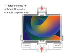
3E. Re-insert the tablet with compatible case. Using your arms, retract the holder in the Y-direction and Z direction until securely fitted.
