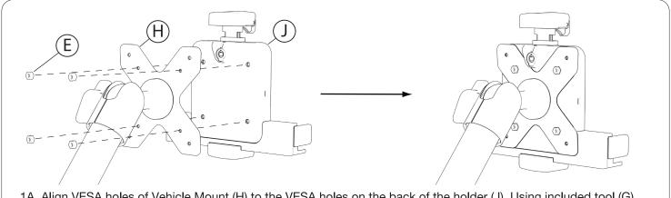
1A. Align VESA holes of Vehicle Mount (H) to the VESA holes on the back of the holder (J). Using included tool (G), rotate in 4 screws (E) until securely fastened.
