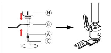
2B. Align the preferred clamp (B) and the vehicle mount (H) and rotate in screw (A) with provided allen key tool (C).
