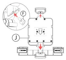
3A. First, make sure the holder is in unlocked position. Insert key (F) to unlock as needed. Using your hands, extend the holder in the Y-direction.
