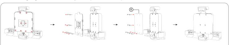
6A. Remove (8) front screws usign a screwdriver (not included) as shown above. Replace front place with component (K) and rotate in screw until securely tightened.
