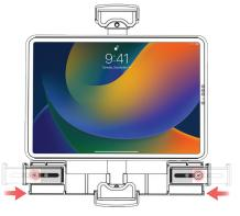
3D. Insert a tablet with compatible case attached. Make sure the two adapters are aligned. Once you insert the tablet with case, it will slide down to let you know it is in the right location. Then, retract the X-direction arms to find the right distance. Remove tablet and use screwdriver to tighten the desired position.
