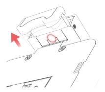
3C. Locate the Z-direction grip arms. On the inside for both the top and bottom, there is a circular button. Press down to loosen the grip arms and extend outwards.
