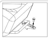
4A. Loosen the bolt (not included) of the seat rail.
