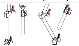
5A. Twist the screw knobs counter-clockwise to release the connection. Adjust the arm to your any preferred position & rotate clockwise until securely tightened.
