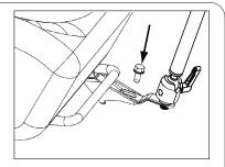
4B. Install the full assembled vehicle mount on the seat rail and screw the bolt back as shown (tool not included).
