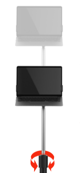
Turn the adjustment knob Counter-clockwise to loose the pole then slide it up and down to desired height and then turn it clockwise to secure it.
