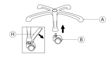
1A. Take one wheel (B) and align it to the leg arm holes on the underneath of the base (A). Initially you can use your hands and manually rotate the wheel until slightly tightened. Then use the provided wrench tool (H) at the hex nut and rotate to securely tighten the rest of
