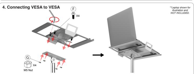
4A. Align VESA Plate (E) to the VESA of the holder (D) Rotate in screws (F) from one side while holding hex nuts (G) from the other end as illustrated. Use provided allen key tool (I) and rotate until securely fastened.
