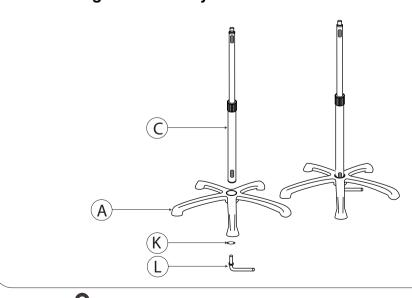
2A. Align the bottom of pole body (C) to the top center of the base (A). While pieces are connected, securely flip over so you can see the bottom. Align washer (K) to the hole on the bottom. Using your hands, identify L-shaped component (L) and rotate through the washer into the hole until securely tightened. Pole body and base should now be securely attached to each
