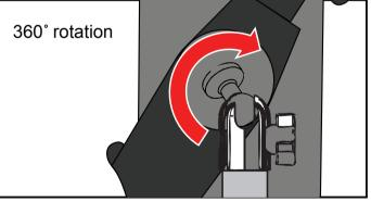
2. Tablet holder rotates 360 degrees for custom viewing angles.
