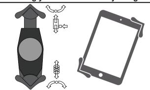
1.Press quick release button on side of tablet holder to release the adjustable end. Insert tablet corner against the spring arm, then push adjustable arm down against opposite corner. Be sure it is as snug as possible.
