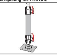
1. Twist the SCREW KNOBS
