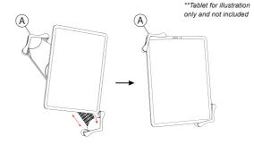
3B. Insert tablet corner against the spring arm. Push adjustable arm down against opposite corner (A). Be sure it is as snug as possible.
