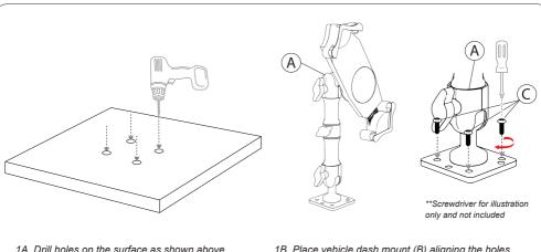
1A. Drill holes on the surface as shown above with power drill tool (not provided).
