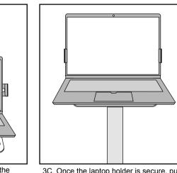
3A. Unlock the holder with the key, and pull out the lock component to allow the holder to adjust.
