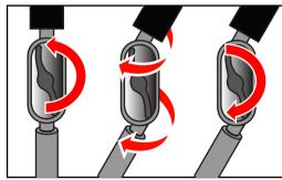
4A. Turn the knob counterclockwise to loosen any of the joints on the vehicle mount. Adjust the arm to the desired angle and position, then rotate clockwise to tighten and secure the position.
