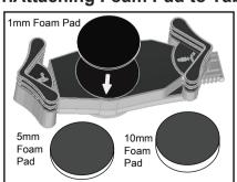
Select the appropriate foam pad according to the thickness of your tablet (or tablet in its case), then press adhesive side into center of the tablet holder. Use this table to determine the appropriate foam pad to use with your tablet.
