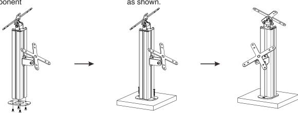
3. Mounting into base creating kiosk. Screw in nails from bottom into base as shown using tools provided .
