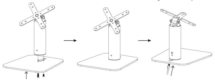
3. Complete the cable routing by pulling cable through the opening and attach to device (below)
