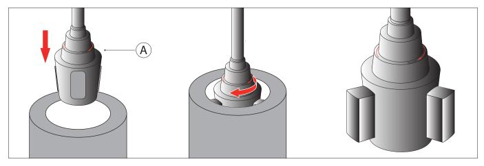
2A. Insert the bottom base of the mount (A) into the cup holder. 2B. Twist the button of the base clock-wise, release the arms to hold it securely.
