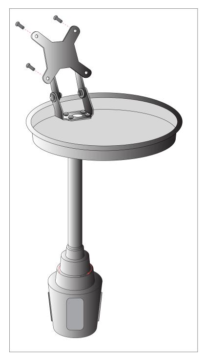
3A. Align VESA bracket (B) VESA holes with the device VESA holes. Rotate in with the provided tool (G) until securely fastened
