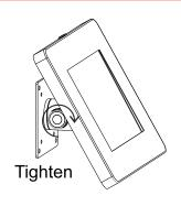
\*Rotate Clockwise to tighten and put the joint in a static state for use.
