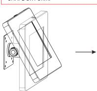
\*Adjust the VESA connection and the object fixed to the VESA to desired tilt and angle
