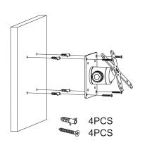
\*Mounting to a Solid Concrete/Block Wall
