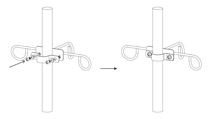
\*After finding the appropriate sized pole, align clamp holes with transfusion holder holes. Then bolt in screws with washer as shown with included allen key tool. Pole is not included, just to be used as an example in the graphics above.
