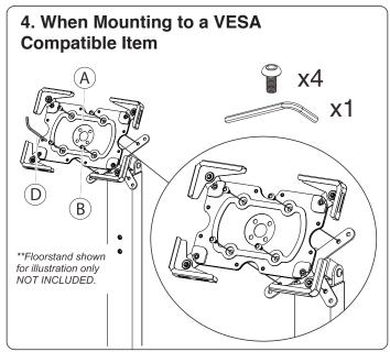
4A. Align VESA holes of tablet holder to that of the VESA compatible item. Rotate from above as illustrated using provided tool (D) and screws (B) until securely fastened. Make sure to do this step BEFORE tablet is inserted.
