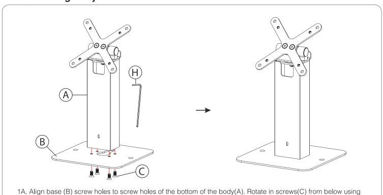
1A. Align base (B) screw holes to screw holes of the bottom of the body(A). Rotate in screws(C) from below using provided tool (H) until securely tightened as illustrated above.
