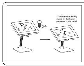
A. Align the holes of the VESA plate to the VESA compatible component. While holding the hex nut in the back of the plate, screw the screws from the front until securely tightened with the provided tools and components.
