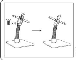
A. Scew in the four screws as illustrated using the provided tools and components
