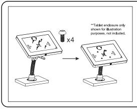
A. Align the holes of the VESA plate to the VESA compatible component. While holding the hex nut in the back of the plate, screw the screws from the front until securely tightened with the included tools and components.
