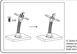
A. Scew in the four screws as illustrated using the provided tools and components
