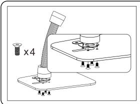
A. Align the holes of the kiosk base plate with the gooseneck. While holes are aligned, screw in the screws with the provided components.
