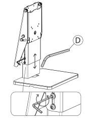
2A. Loosen the side bolt using provided tool (D) to raise or lower to height to your preference. Rotate opposite direction to securely tighten and set your height.
