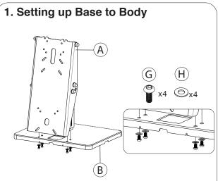
1A. Align base (B) to body (A) as shown. From below, rotate in (4) screws (G) and washers (H) as shown using provided tool (D) until securely tightened.
