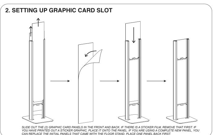
CAN REPLACE THE INITIAL PANELS THAT CAME WITH THE FLOOR STAND. PLACE ONE PANEL BACK FIRST.
