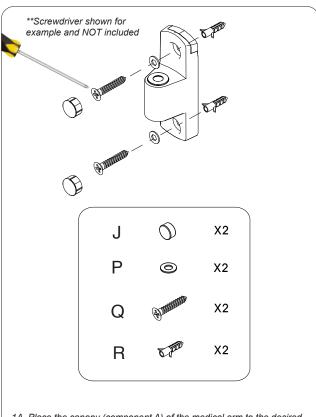
1A. Place the canopy (component A) of the medical arm to the desired location on the wall. Using a screwdriver (not included), and components P, Q, and R - set up the canopy to the wall until securely tightened. Place endcap (component J) on, after everything has been securely tightened for a clean finish.
