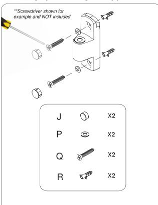
1A. Place the canopy (component A) of the medical arm to the desired location on the wall. Using a screwdriver (not included), and components P, Q, and R - set up the canopy to the wall until securely tightened. Place endcap (component J) on, after everything has been securely tightened for a clean finish.
