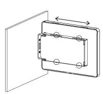
Slide the enclosure to reach ideal position then tighten the screws.
