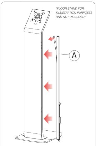
1A. Peel off the 3M adhesive sticker on the back of the LED light bar (A) as illustrated. Attach the LED bar onto the edge of the CTA floor stand (not included) with the wire end on the bottom side. Repeat same steps for the LED bar on the other side of the floor stand
