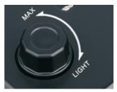
Brightness adjustment knob, the brightness can be adjusted in the brightness range of 5%-100% ,clockwise rotation of brightness is dimmed, counterclockwise rotation is brightness.
