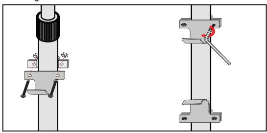
Align hook's screw holes with ring grip's screw holes on opposite sides of pole. Pass screw through holes with screwdriver and tighten nuts on opposite sides as shown in diagram. Repeat for other hook.
