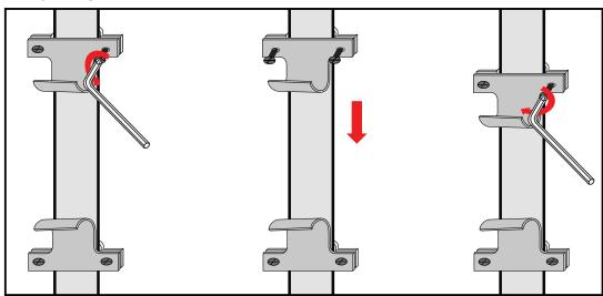
Loosen the screws with the screwdriver, adjust the height or rotate the angle of the hook according to your needs, then tighten the screws again.
