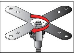
2. Rotate the VESA plate cock-wise to adjust the angle in horizonal .
