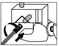
3. To use clamp aligned vertically, screw gooseneck onto the male metal connection bolt on the side of the clamp.
