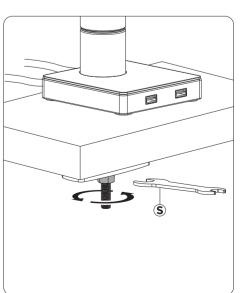
3D. Using provided tool (S), rotate in the hex nut (M) until securely tightened.
