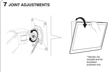
7A. Loosen the joint behind the VESA plate using provided tool. When loose, tilt up and down or rotate portrait / landscape for preferred viewing angles and setup. When done, tighten screw again until securely
