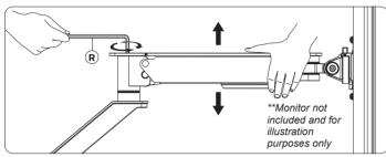
5A. To properly balance the arm with the monitor/device, adjust the spring tension using the provided tool (R) as shown. Make sure the arm is in the horizontal position when making adjustments to avoid damage to the monitor or the mount
