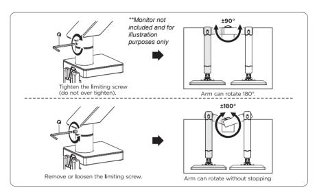
5C. When making swivel adjustments to the arm, use provided tool (Q) at the joint above the mount as shown above. Loosen to allow for swivel rotation as shown. Then rotate clockwise to tighten again once desired rotation has been set for preferred setup.
