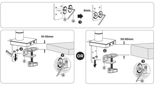
2B. Identify the overall thickness of the surface the clamp will be mounting on. If the thickness is in the 10-55mm range, you will be using the higher setting on the L-shape bracket of the base. If the thickness is in the 50-85mm range, you will be using the lower setting. Rotate in the screws (D) of the bracket until halfway in leaving some space. Hook on the knob component (E). After hooked on, use the provided tool (Q) and securely tighten the screws (D) until securely fastened.
