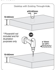
3B. Using drill (not included), drill a 10mm diameter hole for the grommet mount installation. If existing hole is available, make sure diameter is in the 10-60mm range prior to setup for proper installation.
