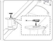
5B. Place cover (H) on top of the joint after finishing with all adjustments with the arm.
