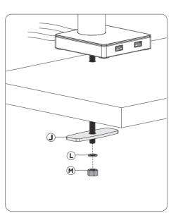
3C. Insert the grommet mount (K) with clamp as shown. Once through the surface, rotate in the rest of the grommet mount components (J, L, M) using your hands initially. Make sure all the components are rotated as far as you can go with no space gaps.
