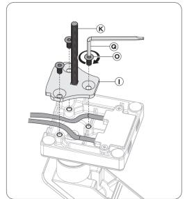
3A. Alight grommet mount (K) with base of clamp mount as shown above. Rotate in screws (O) until securely fastened.
