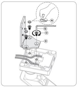
2A. Align L-shape component(D) with base of clamp mount as shown above. Rotate in screws (O) through using provided tool (Q) until securely tighten. Afterwards peel off sticker back of padding (N) and place firmly on the screws
