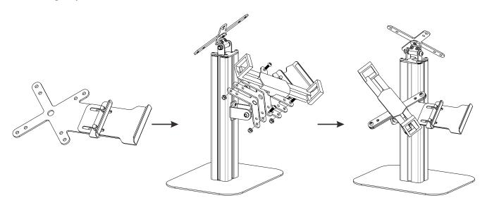
\*Mounting Card Reader Holder on the adjustable joint VESA plate example
