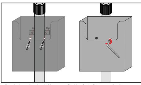
Align grip ring and brochure holder on opposite sides of pole. Pass screws thru holes on inside of brochure holder into holes on grip ring, then tighten nuts on other side. Use Allen key to secure.
