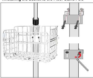
Align grip ring screw holes with basket screw holes on either side of the central pole. Pass screw through washer, then through screw hole, and attach nut on opposite side. Use Philips Screwdriver to tighten. Repeat for other screw.
