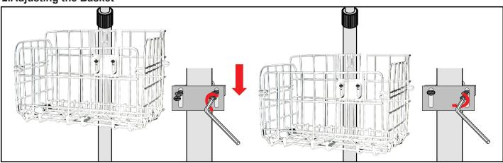
Loosen the screws with the screwdriver, adjust the height of the basket, then tighten screws again.
