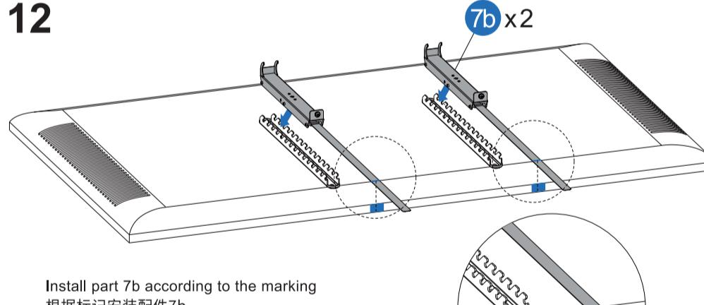
Install part 7b according to the marking
