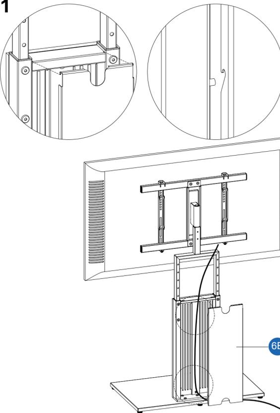
EN Select appropriate screws from M-A to M-G and install part # 4 on the four screw holes on the back of the TV. The back of the TV is flat, and the A1 installation method without gasket can be used; If the back is uneven, A2 installation method with washers (M-H to M-J) can be used, and thick washers can be superimposed according to the situation.
