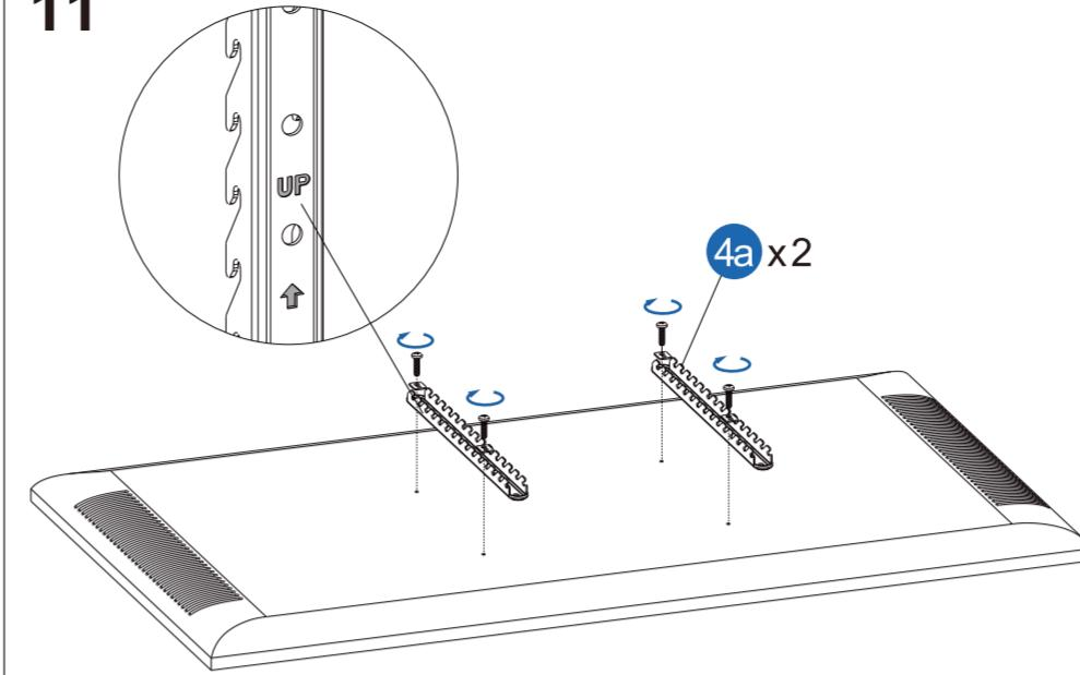
EN Select appropriate screws from M-A to M-G and install part #4a on the four screw holes on the back of the TV. The back of the TV is flat, and the A1 installation method without gasket can be used; If the back is uneven, A2 installation method with washers (M-H to M-J) can be used, and thick washers can be superimposed according to the situation.
