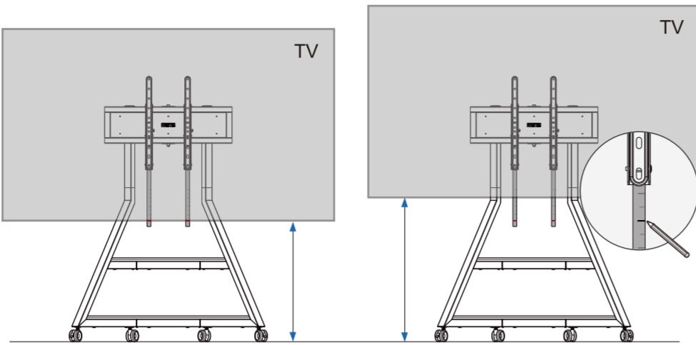
The adjustable range of the distance from the bottom of the TV to the ground is marked on the part 4, so that you can choose the appropriate height. You can choose the height, make a mark on the ruler, and then disassemble and install the part 4 to the back of the TV.
