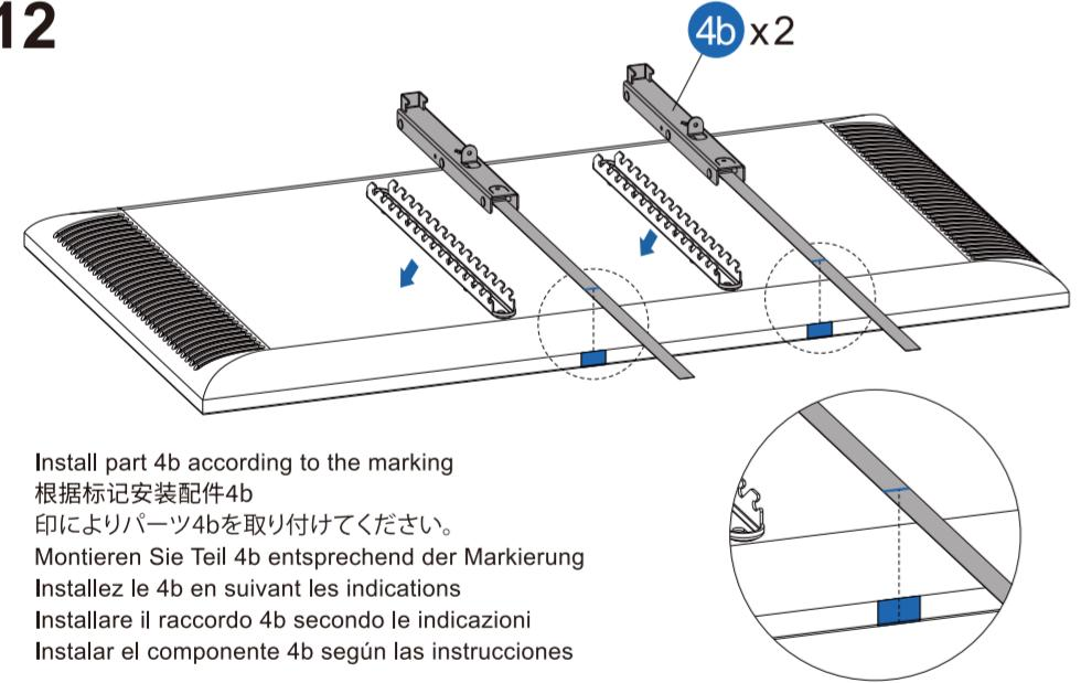
Install part 4b according to the marking
