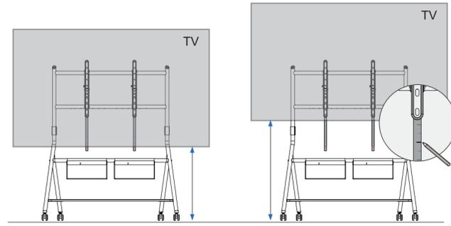
EN The adjustable range of the distance from the bottom of the TV to the ground is marked on the part 7, so that you can choose the appropriate height. You can choose the height, make a mark on the ruler, and then disassemble and install the part 7 to the back of the TV.
