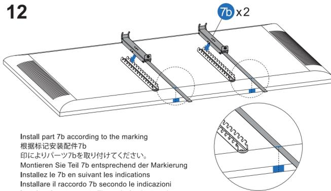
Install part 7b according to the marking
