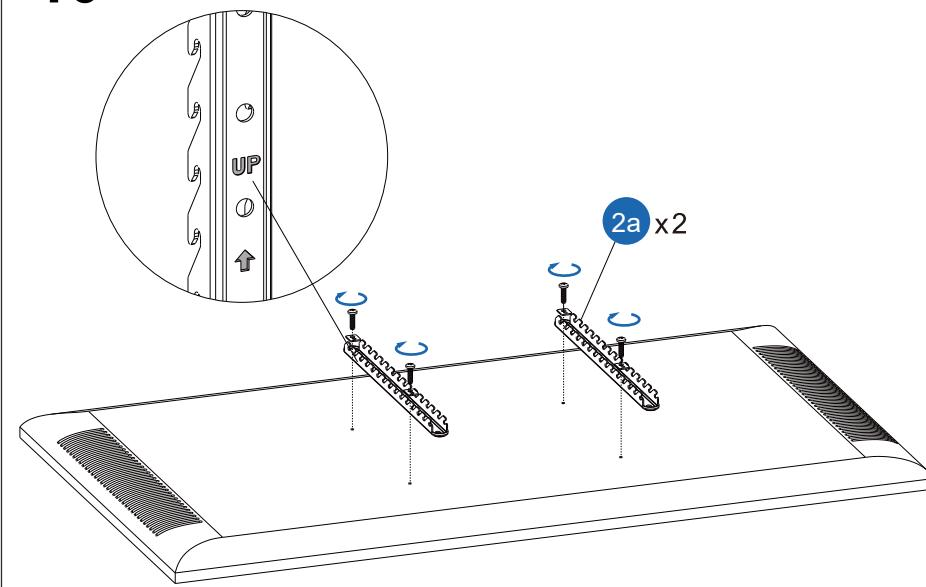
**EN** Select appropriate screws from M-A to M-G and install part #7a on the four screw holes on the back of the TV. The back of the TV is flat, and the **A1** installation method without gasket can be used; If the back is uneven, **A2** installation method with washers (M-H to M-J) can be used, and thick washers can be superimposed according to the situation.
