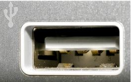
Plug the USB into the port and make sure it is full inserted. If your computer does not have a port which looks similar to the picture (it may be flipped or a different color), then you may need to use a serial cable instead.
