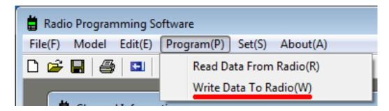
A new window should appear. Make sure your radio is plugged in, turned on, and your COM port settings are correct. Click **Write** and wait for the **Finished** message to appear. Do not unplug the radio or close the window until the message appears. You can close the window by clicking **OK**.
