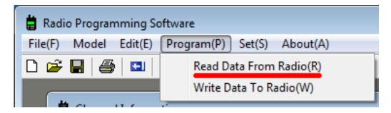
Click on **Read** and the loading bar should start moving. If it does not, make sure it is properly plugged in (and your COM port settings are correct) Do not unplug the radio, or close the window, while it is reading. Once it is done you can click on OK to close the window.
