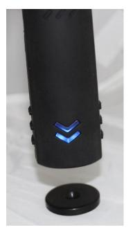
**Note:** Metal will interfere with the RFID scanning. Make sure no metal is in-between the scanner and the tag. Also make sure that you do not have other RFID tags near the one you are trying to scan, as this will also make the scanner fail to scan.
