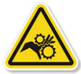
Machinery Pinch Point
