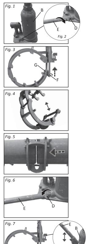
**1.** Release all pressure from hydraulic cylinder (*B*, *Fig.* 1) by turning release valve. (*D*, *Fig.* 2) Note: Use hydraulic handle (*E*).
