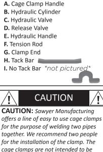
cage clamps are not intended to be used as sole support of the pipe nor to lift the pipe. These clamps are not designed for the use of tees, elbows, valves or other fittings. After each use clean and store in a warm, dry area.
