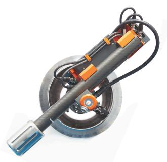
The Bevel360 Mk 2 eliminates doubt about bevel compliance, helping clients achieve better fit-up, improve weld quality and install higher quality pipelines. State-of-the art laser sensors provide a comprehensive weld profile in c. 20 seconds, allowing welding to proceed efficiently. The updated Mk 2 version was launched in 2023, with several major improvements such as wireless power and compatibility with OMS SmartFit.
